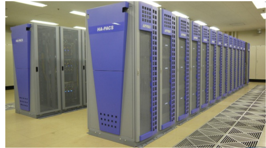
HA-PACS (268 node), 2012 Appro, Intel SDB, NVIDIA M2090 Peak 802TFLOPS HPL 421.6 TFLOPS (#41 in TOP500, 2012/06)
