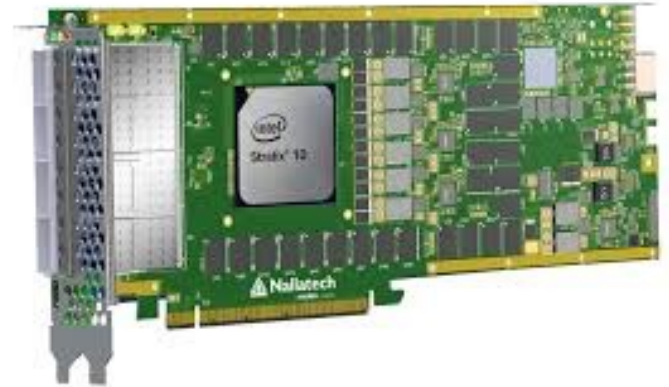
BittWare 520N with Intel Stratix10 FPGA equipped with 4x 100Gbps optical interconnection interfaces
