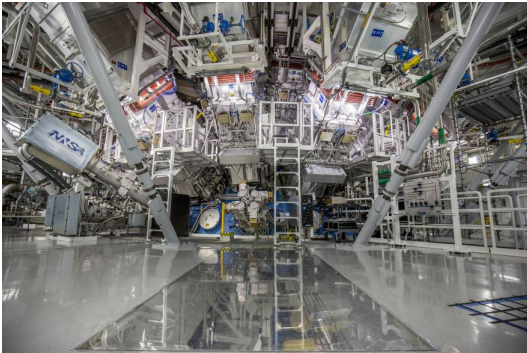
The target chamber of LLNL's National Ignition Facility, where 192 laser beams delivered more than 2 million joules of ultraviolet energy to a tiny fuel pellet to create fusion ignition on Dec. 5, 2022.
