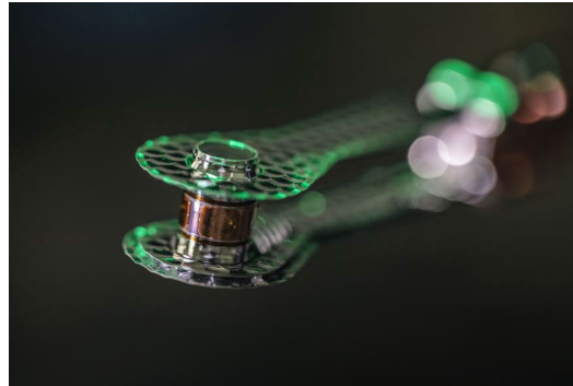
The hohlraum that houses the type of cryogenic target used to achieve ignition on Dec. 5, 2022, at LLNL's National Ignition Facility.
